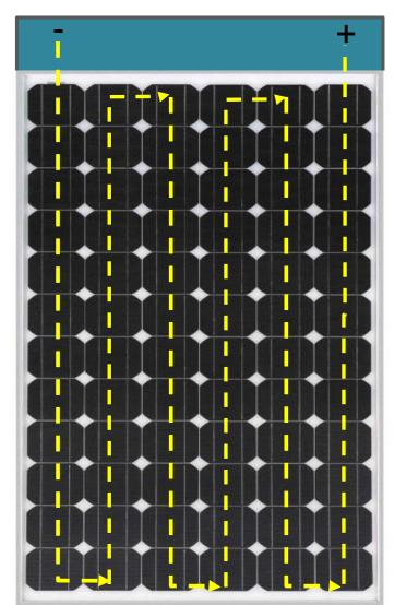
Like batteries in a flashlight, individual solar cells are connected in series
