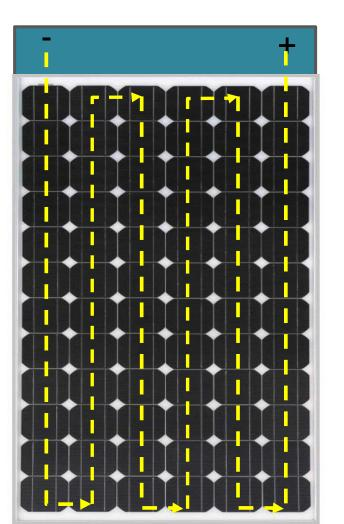
Think of shading like a flashlight with three new cells and one old one. Current flows from high to low, so in the same way that the old battery becomes a drain on the others, the shaded solar cell becomes a consumer of electricity, not a
