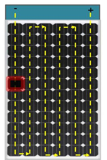
To prevent this, by-pass diodes are wired in parallel with the solar cells and become a lower resistance path around the shaded cells
