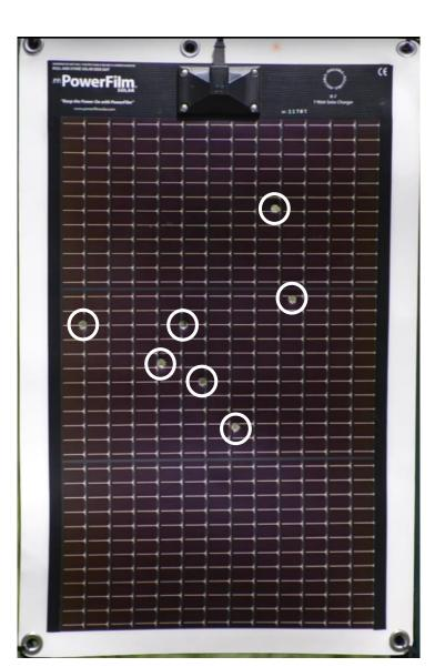
...only resulted in a loss of less than 20%
