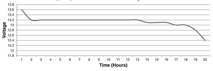
• A 40 ah LiFePO4 battery can provide 40 amps for an hour and can still be recharged
