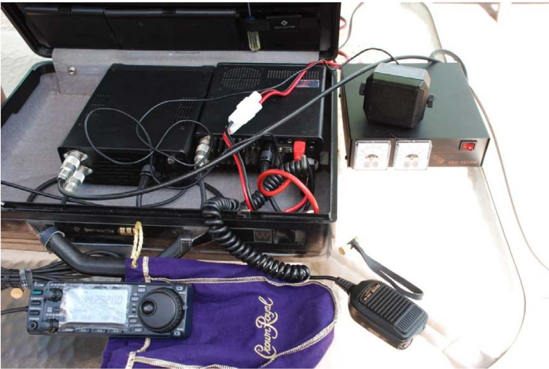
Hook up the power source. We added Anderson Powerpole connectors to the 706 power cord allowing rapid attachment to any source of 12VDC with matching connectors. We also have a Hi Amp Cigarette plug adapter and battery clamps which would allow us to power off of a vehicle or car batteries. Here we are using a Samlex SEC1235M switching power supply.
