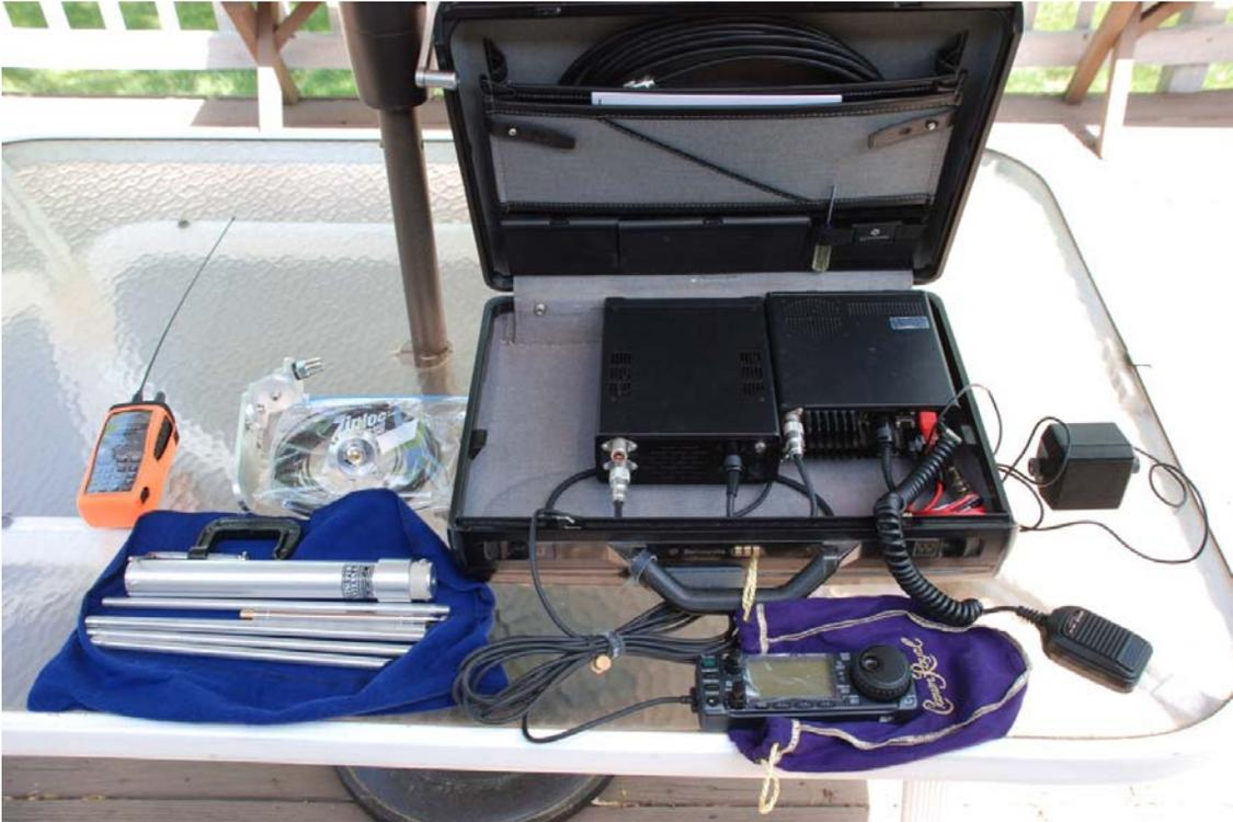
To place the station in operation, remove the antenna package, HT, remote control head microphone and speaker.
