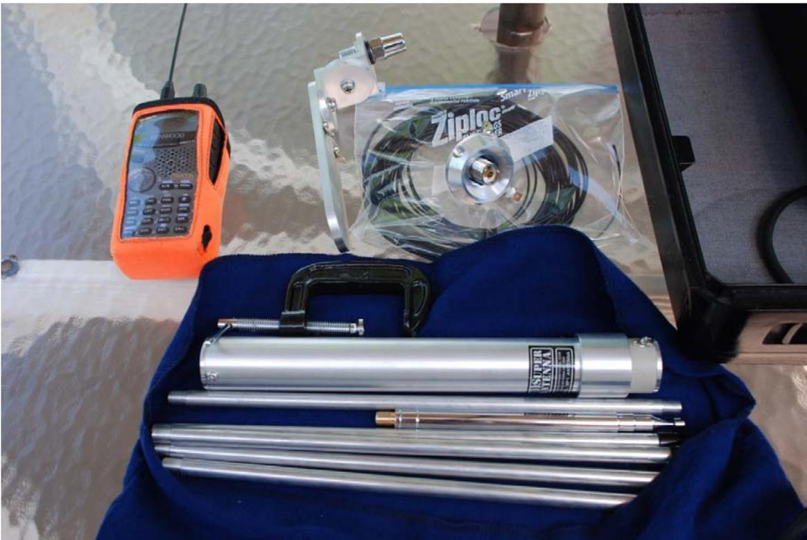
Assemble and erect the antenna. In our kit we have a SuperAntennas MP-1, a very compact 40m to UHF antenna kit. It works like a screwdriver antenna without the screwdriver motor. The machined aluminum parts thread together easily with no tools, and the antenna can be clamped to a rail or other structure or you can buy the optional tripod for free-standing operation. An optional 80m coil is also available..
