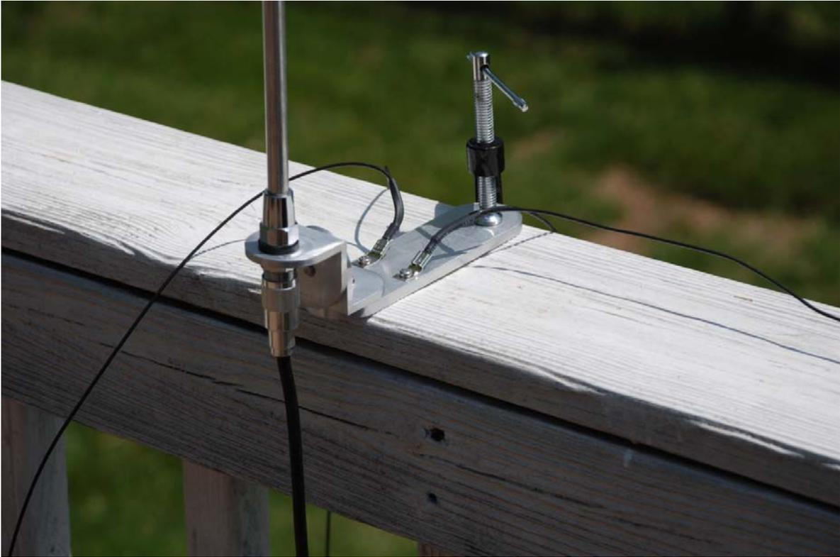
The MP1 base with wire radials attached is easily clamped to the railing on our deck with included C-clamp.
